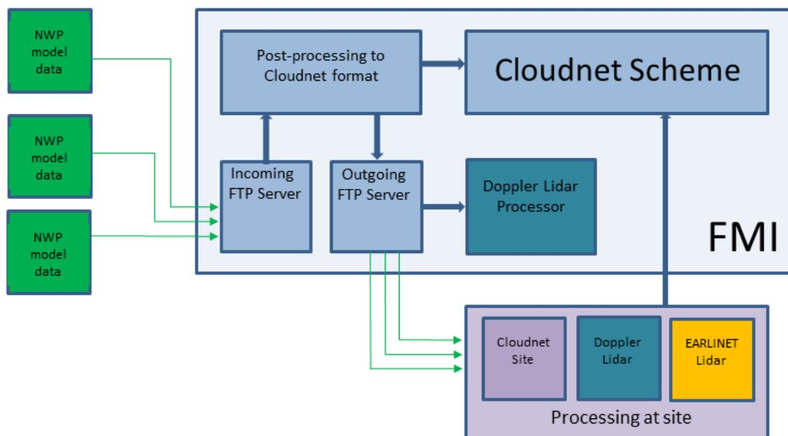
**Figure 3:** Model data workflow within Cloudnet
